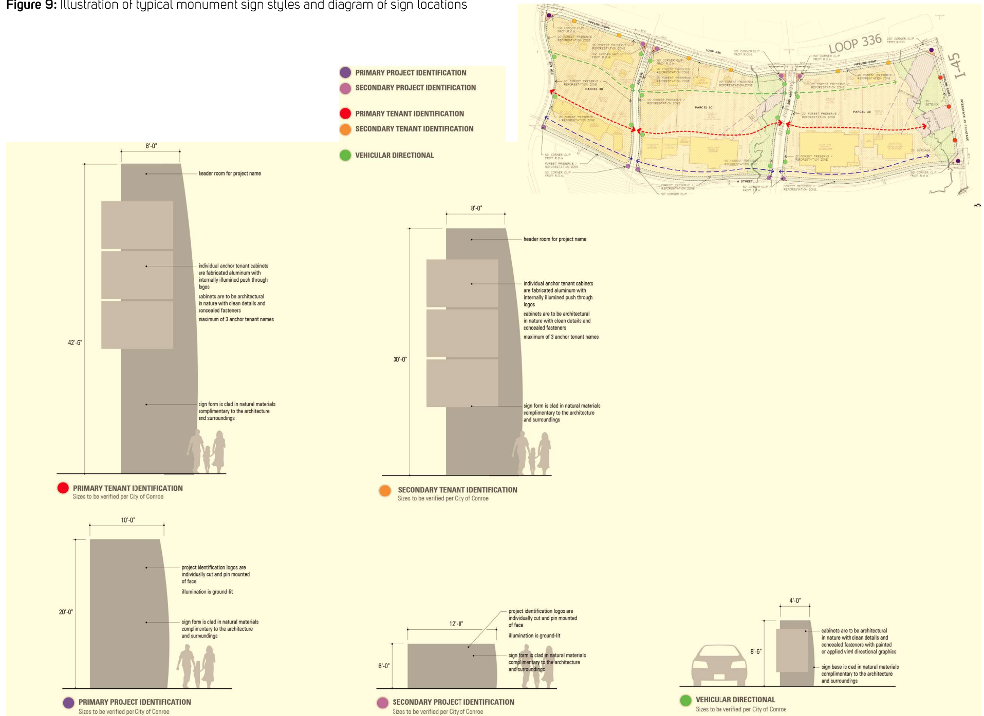
Figure 9: Illustration of typical monument sign styles and diagram of sign locations
